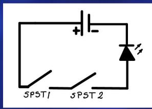
3. The circuit below represents the action of a logic gate. A switch in the "ON" position corresponds to 1, and "OFF" corresponds to 0. The LED being "ON", represents 1, and it being "OFF" represents 0. Which logic gate is represented by this circuit?
