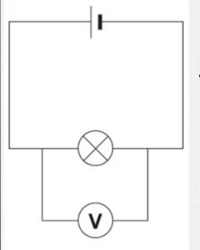
Voltage measurements must be done <u>in</u> <u>parallel</u>
