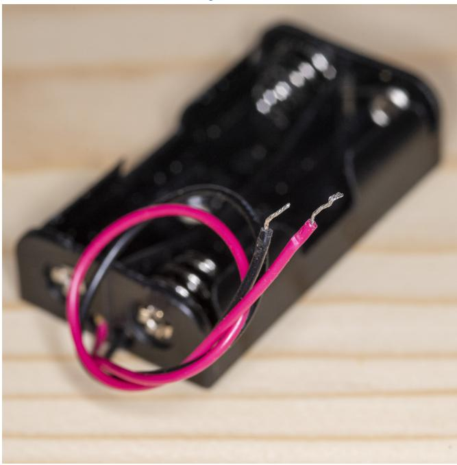
The wires on the battery holders from previous years are tinned threaded wires – they're flimsy. These *do* work with the terminal blocks:
