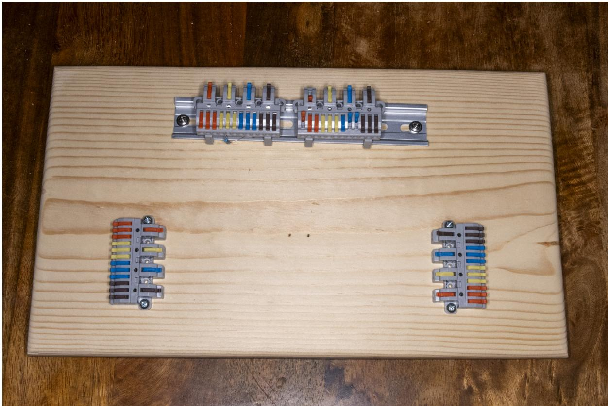
These are simple 1x10 boards with a piece of DIN rail and some lever-lock terminal blocks installed.
