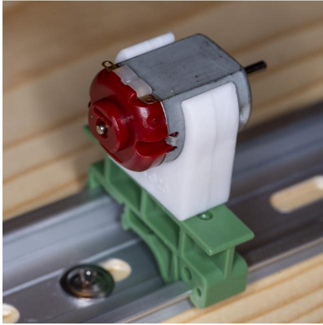
Please be careful with these – they will turn when exposed to electricity! The wheels or fan blades should be used with the motors so it's clear to the students when the motor is turning (and they will slow the shaft down).
